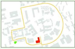
The Old Power House is shown in green; in red is the building that houses Cal Poly's heating and cooling plant #4 (Engineering South, #40). The Utilidor, a mile-long vault under sidewalks that delivers hot water, chilled water, and drinking water, is shown in orange.
