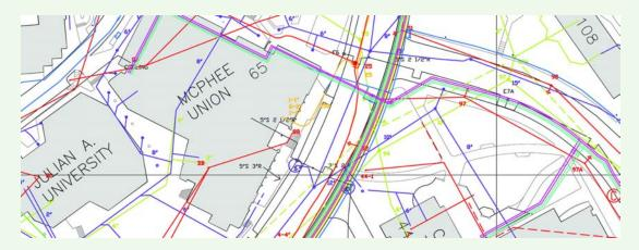
Current computer database, Atlas B. Atlas B shows it all, useful for digging and avoiding unpleasant surprises. Here the colors are simplified. Blue indicates water. Purple indicates storm drains. Cyan indicates chilled water.
